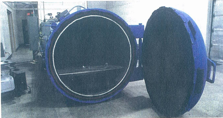
Allflight, an Infinity Air company, uses this autoclave to cure parts in its composite metal bonding facility.
